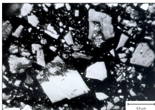
Fig. 7. Loss of pyrite mass in favour of secondary minerals
