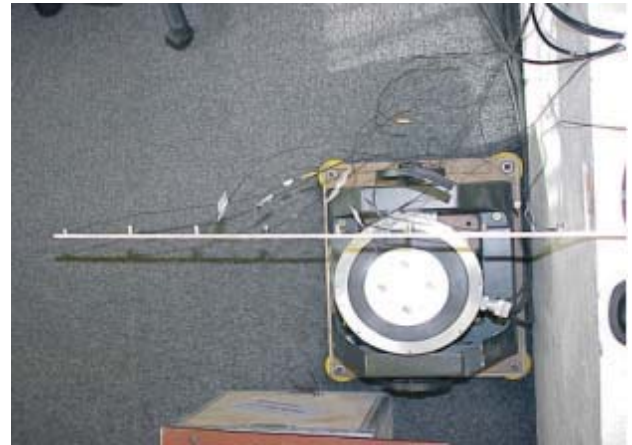
Fig. 5. Laboratory stand for investigations of free vibrations of damped beam
