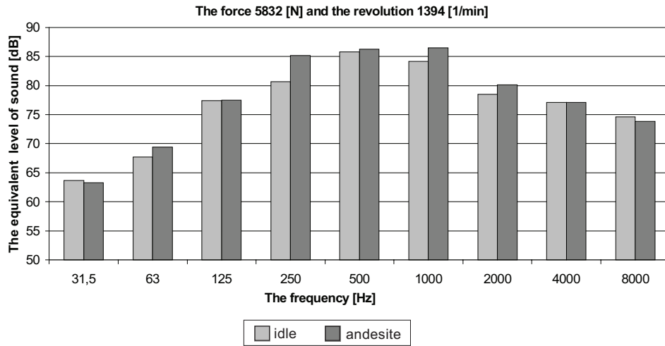
Fig. 10. The comparing of equivalent levels of sound at various frequencies in idle mode and during andesite disintegration
