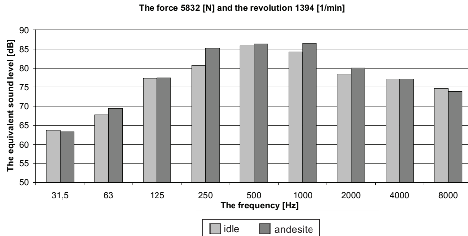
Fig. 13. The comparing of equivalent levels of sound at various frequencies in idle mode and during granite disintegration
