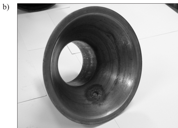
Fig. 12. Measurement section of the diffuser-pipeline system (a); diffuser (b); diffuser with two flow guides (c)
