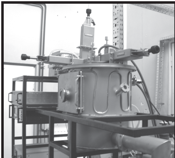
RYS. 2. Widok systemu MW/RF PCVD. FIG. 2. A view of the MW/RF PCVD system.
