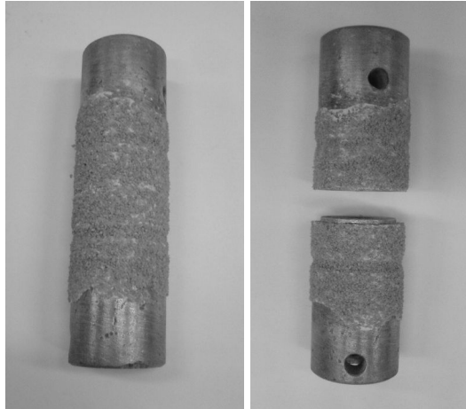
Fig. 2. Divided sample of a roll shape after deposition of the ceramic layer, before and after the rupture
