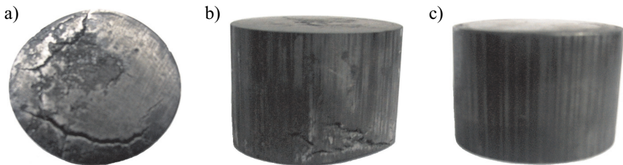
Fig. 1. Shape of samples obtained in closed-die hot compaction of Al17Si5Fe3Cu1.1Mg0.6Zr powder: a) temperature 500 ^{\circ}\text{C} , punch unit pressure 50 MPa; b) 400 ^{\circ}\text{C} , 150 MPa; c) 450 ^{\circ}\text{C} ; 150 MPa
