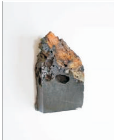
Fig. 13. The crystal structure of the section of a slag block from Garbacz–Skala (No. 57) under a brick that fell into liquid slag
