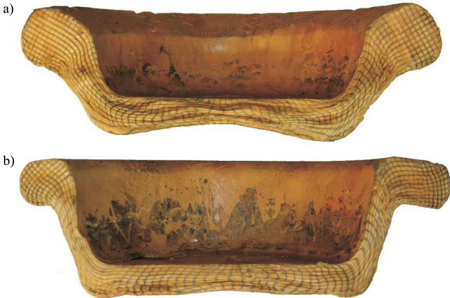
Fig. 3. Physical modelling of a three-stage forging process: a) blocker; b) finisher
