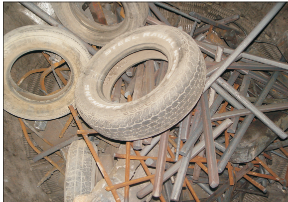
Fig. 4. Charging of scrap tires in scrap basket
