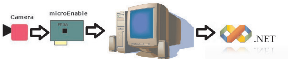
Fig. 6. General schema of the vision system connections
