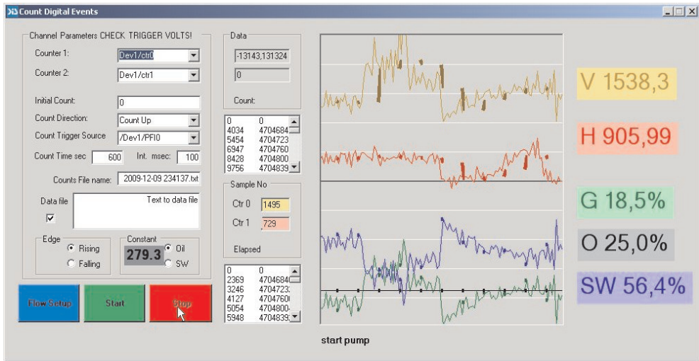
Fig. 6. Example of gamma radiation measurements while pump start in a flow rig. Rig filling: 50% sea water, 25% Diesel oil
