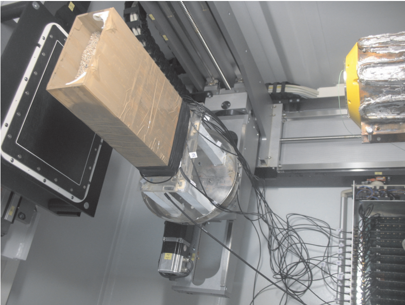
Fig. 8. The simultaneous measurement of silo flow by ECT and X-ray tomography systems
