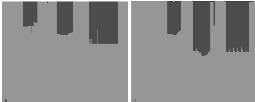
Fig. 3. Reconstruction of obstacles location calculated from disparity distribution. Left picture: from original images, right picture calculated from images with different obstacles location (stereo pictures not included)
