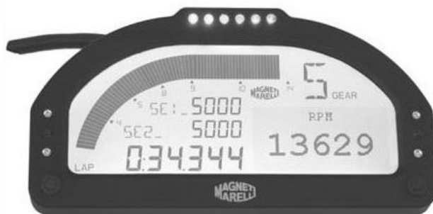
Fig. 2. The device MDU230 company Magneti Marelli [4]
