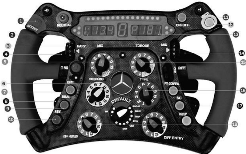
Fig. 1. View Racing Wheel integrated with the dashboard [3]: 1 – BOOST, 2 – LAP TIME, 3 – HARVEST, 4 – DOWNSHIFT PADDLE, 5 – MIX, 6 – BITE POINT, 7 – BPF, 8 – CLUTCH PADDLE, 9 – BBAL, 10 – REVERSE GEAR, 11 – SHIFT LIGHTS, 12 – LIMITER, 13 – ENGINE PARAMETERS, 14 – UPSHIFT PADDLE, 15 – TORQUE, 16 – TYRE, 17 – CLUTCH PADDLE, 18 – DIFFERENTIAL
