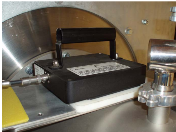
Fig. 4. Beryllium neutron activation counter dedicated to the PF-24 device.
