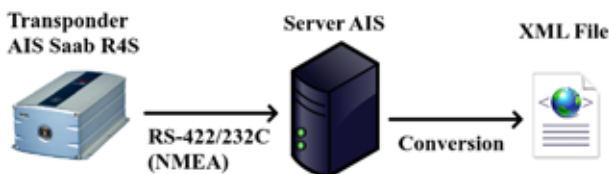
Figure 3. AIS data system architecture
