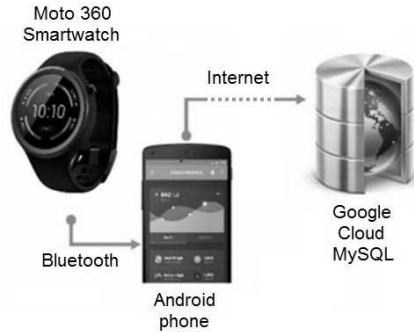
Fig. 12. Connectivity of the smartwatch with Android and cloud.
