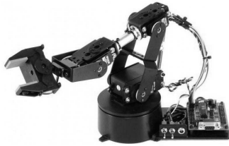
Fig. 10. AL5A robotic arm with SSC-32 controller board [25]
