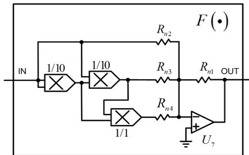
Figure 12. Designed electronic circuit modeling of the inverting hyperbolic sinusoidal block. Here the values of components are selected as:  $R_{n1} = 10k\Omega$ ,  $R_{n2} = 1M\Omega$ ,  $R_{n3} = 60k\Omega$ , and  $R_{n4} = 120k\Omega$
