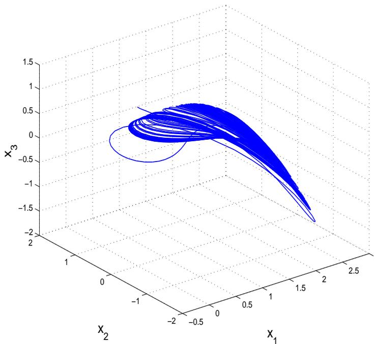
Figure 1. Strange attractor of the Sprott jerk system
