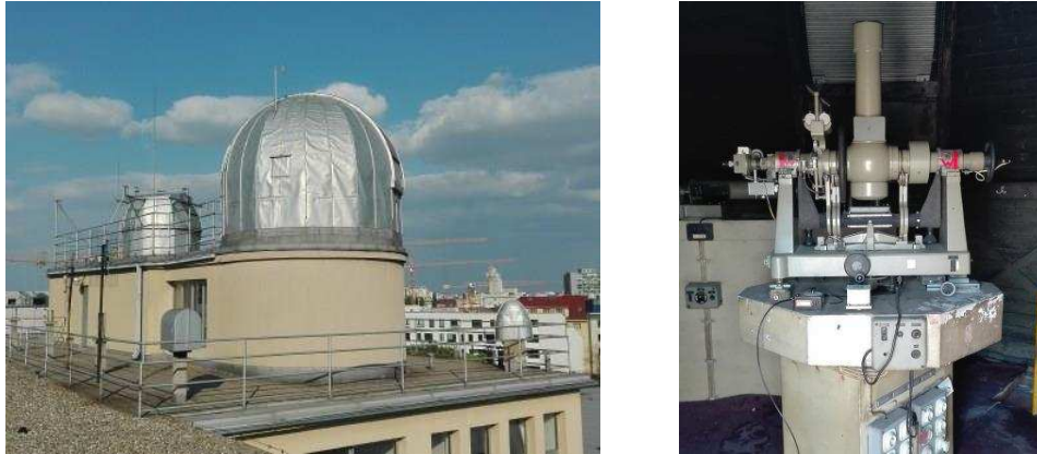
Fig. 3. Pillar for geodetic astronomy observations situated on top of 5-floor historical building of SUT in Bratislava. Inclination sensor is on the pillar in front of the Transit Instrument.
