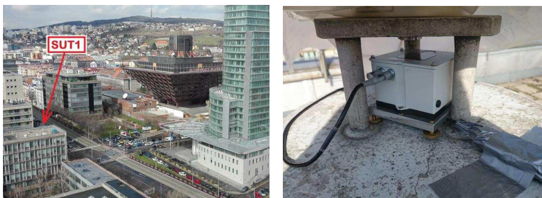
Fig. 2. Pillar monument of GNSS station SUT1 situated on a top of 6-floor building of Faculty of Civil Engineering in centre of Bratislava.
