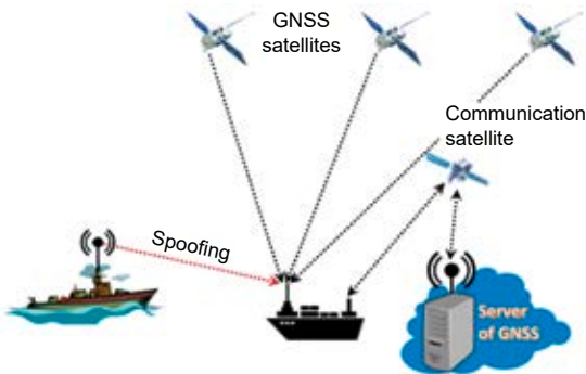
Figure 6. Spoofer broadcasts signals of the visible part of the GNSS satellite constellation (C) or broadcasts simulated GNSS signals (D)
