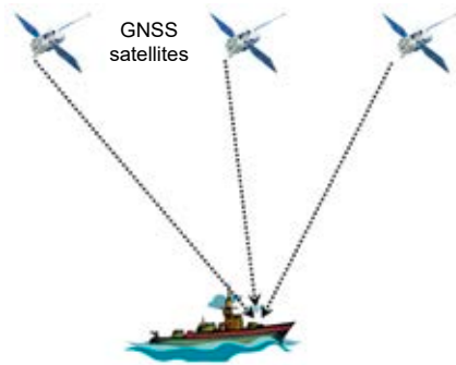
Figure 5. Spoofer records signals of the visible part of the GNSS satellite constellation
