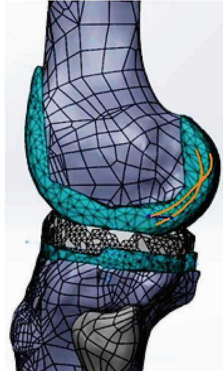
Fig. 12. Sagittal view of the knee model with prosthesis: the “carriage” (blue) is shown on the insert and the two paths (orange) on the femur component
