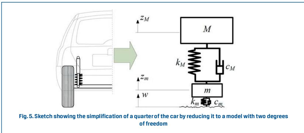
The model of the vertical dynamics of a motor car suspension system was described by a pair of second-order differential equations of motion:
