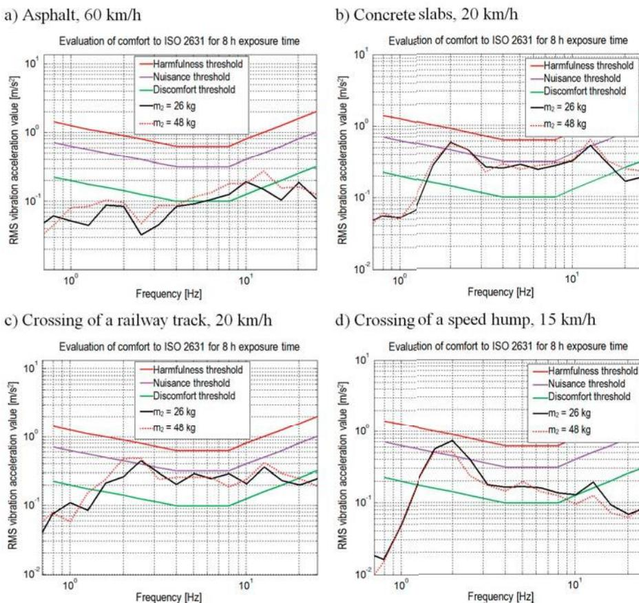
**Fig. 4. RMS acceleration values of vertical car body vibrations above the rear axle in 1/3 octave frequency bands from 0.63 Hz to 25 Hz for selected vehicle operation conditions, against the standard limit values according to ISO 2631 for 8 hour time of exposure to vibrations**
