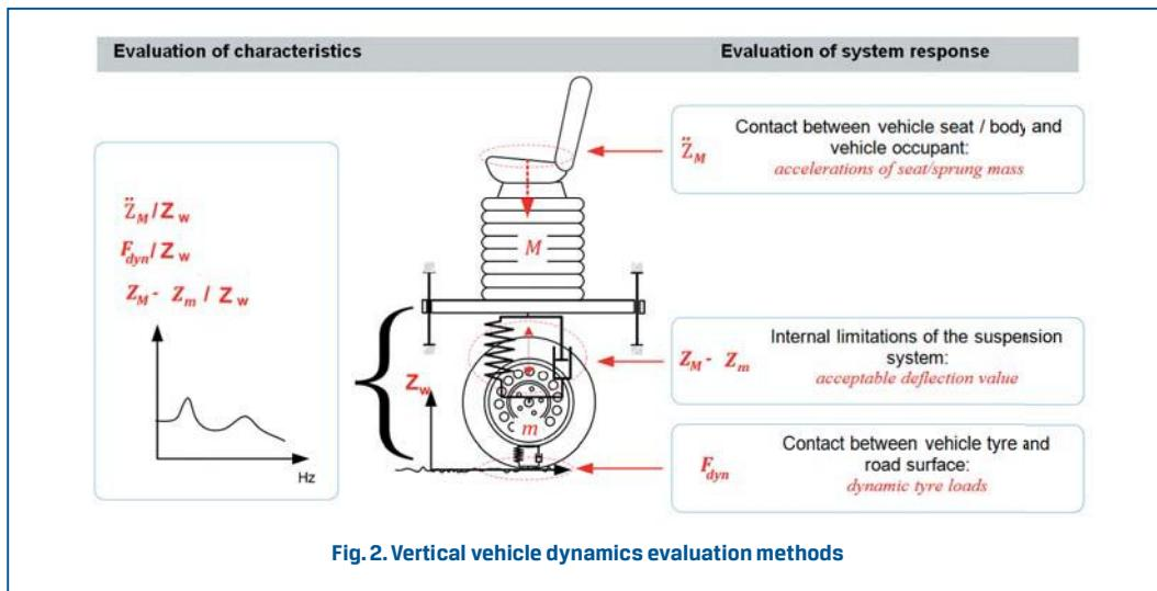
In the former case, the evaluation must be carried out for specific inputs (i.e. specific vehicle operation conditions defined by kinematic inputs depending on the type of road surface roughness and the speed of vehicle drive on this road surface), by evaluating the vehicle occupant accelerations as a comfort indicator and dynamic wheel loads as a safety indicator.
