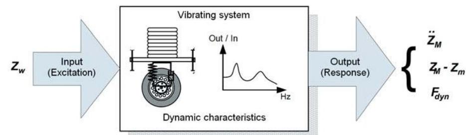
**Fig. 7. Quarter-car suspension system as a dynamic system**
