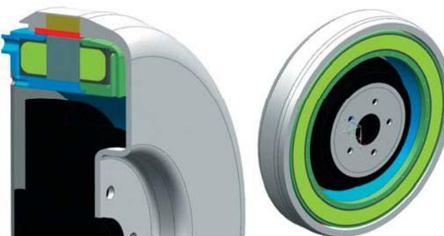
Fig. 1. A concept of the in-wheel electric motor
