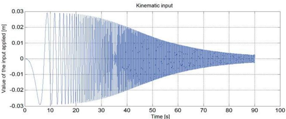
**Fig. 6. Kinematic input function used to examine dynamic system characteristics**
