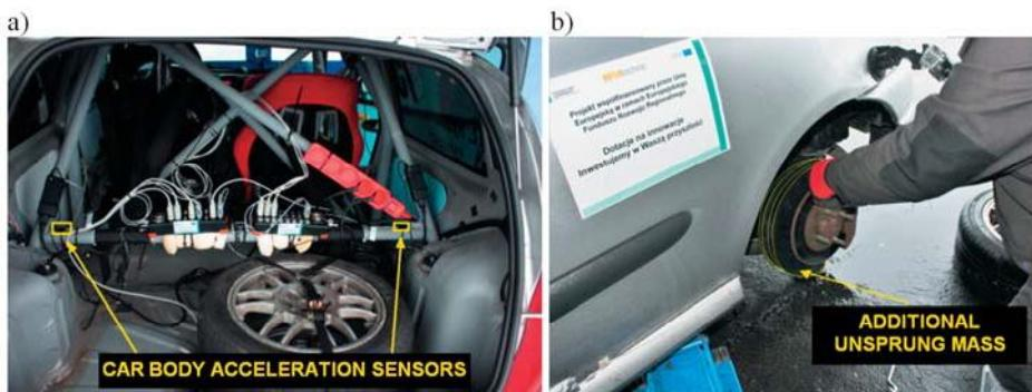
**Fig. 3. The test car Renault Clio II: a) Locations of the rear vehicle body part acceleration sensors; b) Location of the weight (non-revolving) that represented the extra unsprung mass**
