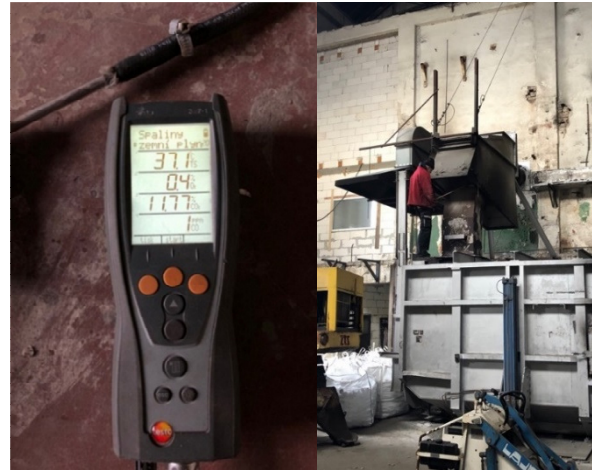
Fig. 4 Measurement of pollutant content produced during melting of Al alloy in the gas melting furnace KOV 010/1998 using Testo 340 measuring equipment
