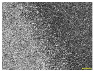
**Figure 1** Structure of the weld made using Union X90 welding electrode and a shielding gas mixture Ar + 10% CO,
