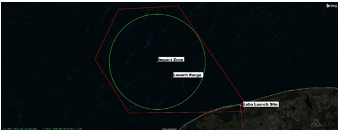
Pic. 5. Launch range zone and launch corridor of NEO Suborbital Mission. Green – impact zone. Red – launch range zone. Purple – launch site.
