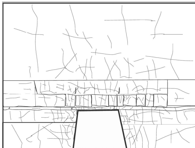
Fig. 1. Roof falls in mining sidewalks, a) roof falls between rockbolts (fot. K. Skrzypkowski), b) roof block separation above the rockbolts (photo: D. Juszyński)
