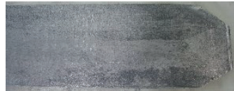
Fig. 4a. the strip of sheet AlMn1Cu alloy before the 1 st pass
