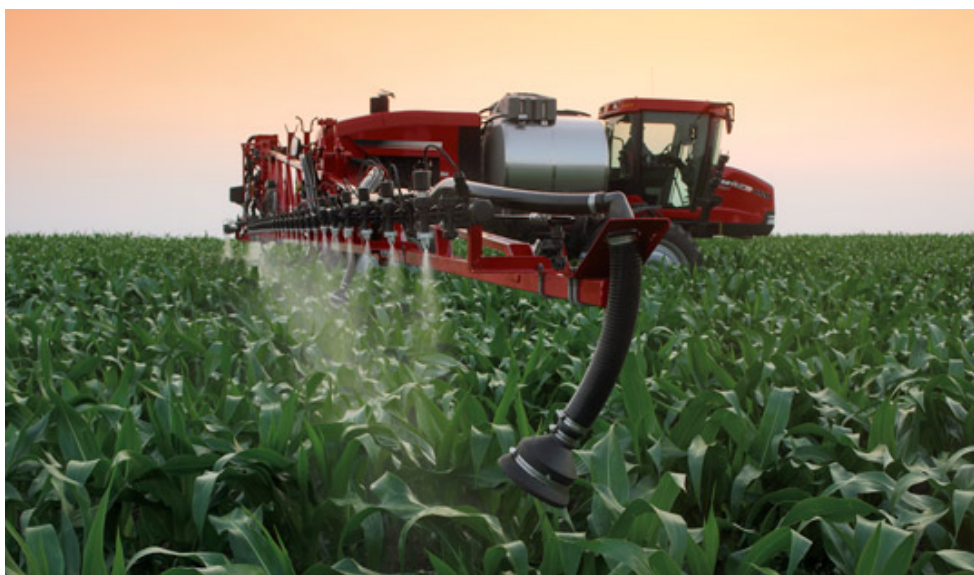
Figure 5. Corn spraying using satellite system (multispectral radiation analytical channels combined with the GPS system) for application of fertilizer of Case Co.
