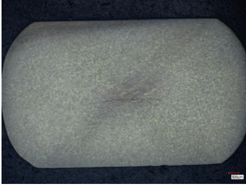
Fig. 1. An example of wire cross-section etched with Nital with a HIC near the centreline. Etching reveals a "X" pattern near diagonals related to plastic deformation during the cold rolling process
