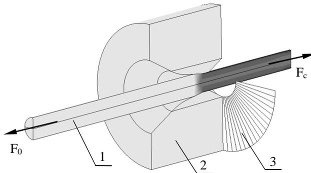
**Fig. 1. Scheme of drawing process modelled: 1 – drawn wire, 2 – drawing die, 3 – abutment surface,  $F_c$  – drawing force,  $F_0$  – backpull force**
