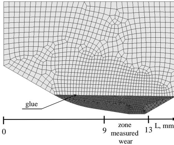
**Fig. 3. FEM Model of tool and zone of the measurement his wear**
