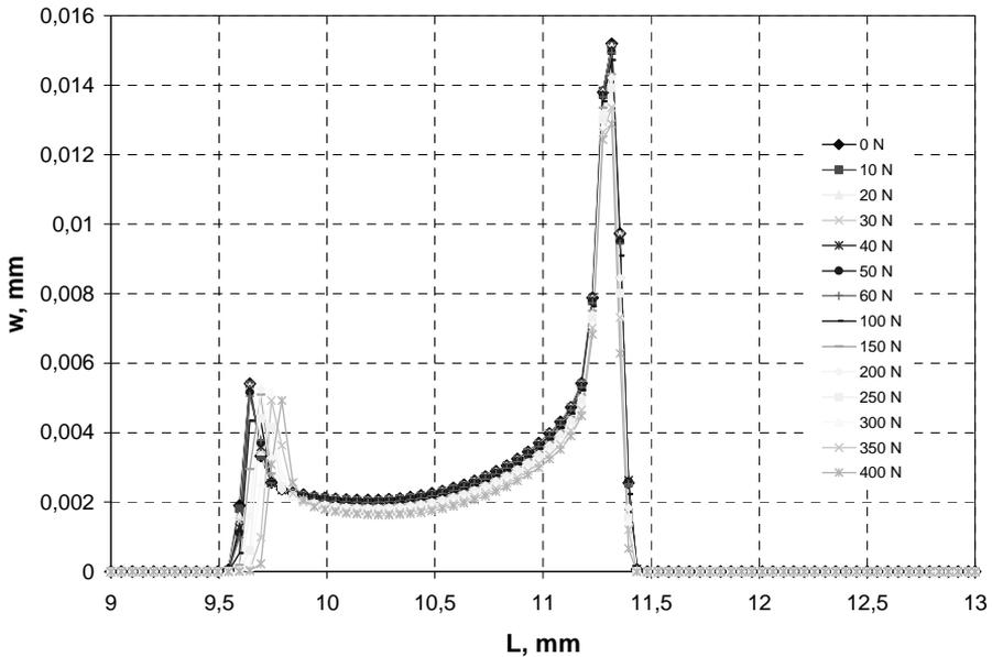
**Fig. 4. Change of wear of drawing dies on their length**
