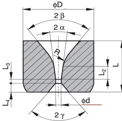
**Fig. 2. Dimensions of drawing die for investigations:**  $\phi d = 3 \text{ mm}$ ,  $\phi D = 20.45 \text{ mm}$ ,  $R = 10 \text{ mm}$ ,  $2\beta = 2\gamma = 60^\circ$ ,  $2\alpha = 18^\circ$ ,  $L = 17 \text{ mm}$ ,  $L_2 = 5.2 \text{ mm}$ ,  $L_3 = 1.5 \text{ mm}$ ,  $L_4 = 3.2 \text{ mm}$
