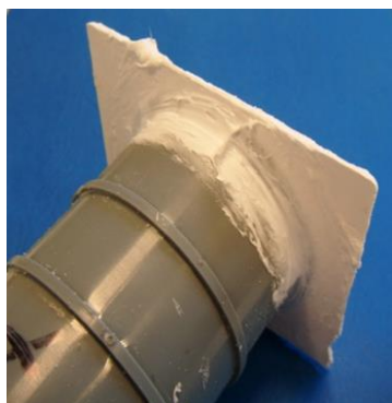
Fig. 4. Sampler with glued ceramic mould readied for permeability tests
