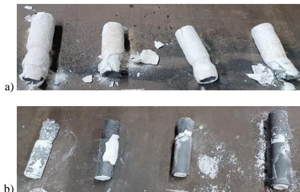
Fig. 8. Test castings subjected to knocking-out on vibratory table – external side of bushing casting: a) view of castings after 1 mammoth treatment on vibrating table; b) view of castings after 3 mimytes processing on vibrating table
