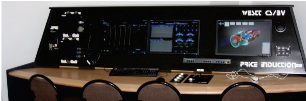
Fig. 3. The engine test bench WESTT CS/BV in the front view, measurement data is displayed on the screens
