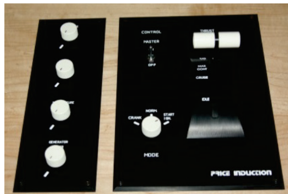
Fig. 4. The control potentiometers and flying controls; the switches at the flying controls are used to start the virtual engine
