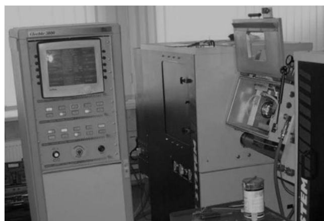
Fig. 5. Physical simulator Gleeble 3800, used in experimental research
