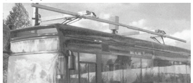
Fig. 2. Bus being charged with use of the pantographs en route.
