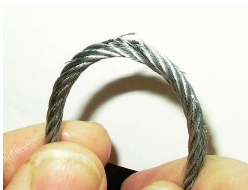
Fig. 2. The damaged cable KSAN 3,5 removed from the aircraft
