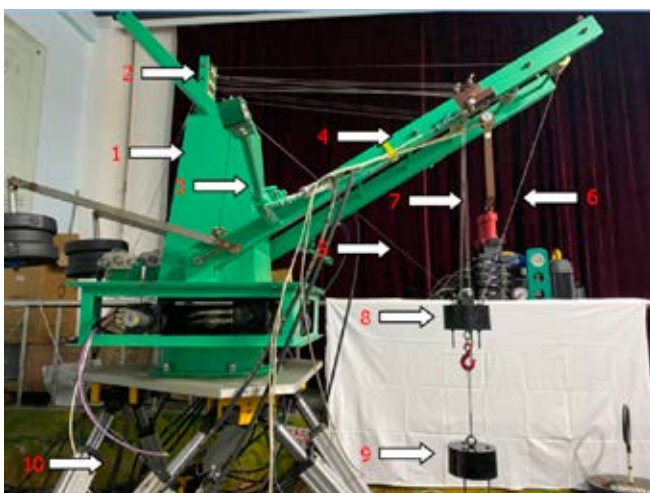
1 - Crane body, 2 - Pulley set, 3 - Folding arm, 4 - Crane boom, 5,6 -Auxiliary cables, 7 - Main cable, 8 - Primary pendulum, 9 - Secondary pendulum, 10 - 6DOF platform
