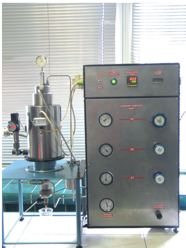
Fig 3. Apparatus for analyzing gas migration through bonding cement slurry in wellbore-like conditions
