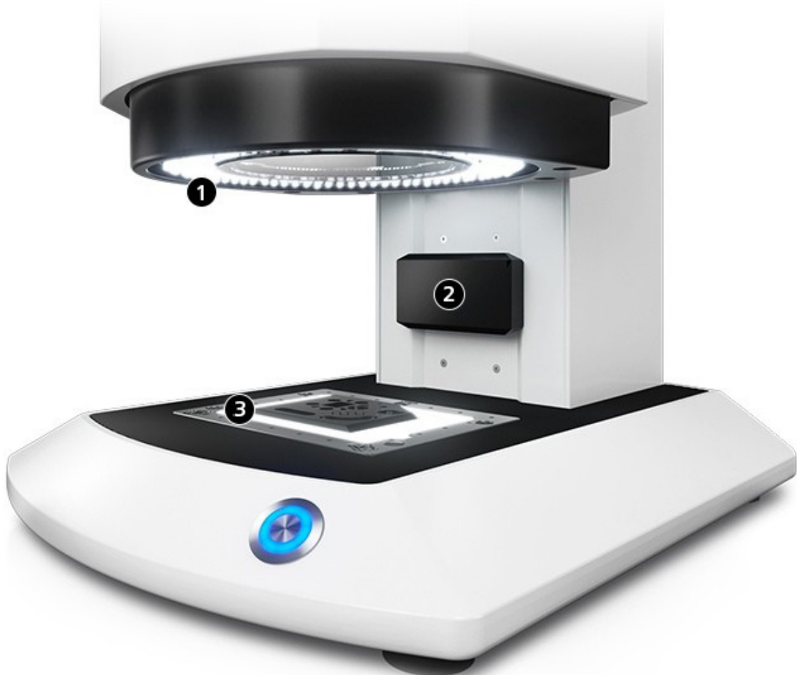
Fig. 2. (1) Eight-segment double ring light for variable reflected-light illumination (2) Mounting block for optional coaxial light (3) Transmitted light for maximum contrast
