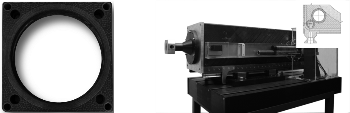
Fig. 1. Experimental composite spindle ram (Composite body – left; spindle ram with connection interfaces-right)
