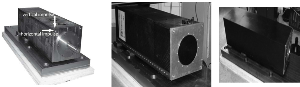
Fig. 8. Experimental modal analysis of clamped experimental spindle rams (left – steel spindle ram II with denoted points of excitation; centre - composite spindle ram, right – hybrid spindle ram)
