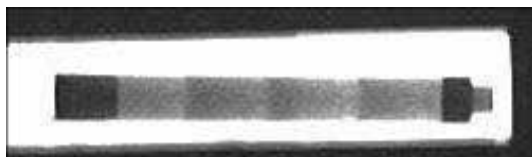
Figure 3. Real Time Rentgenoscopy image of tested multi-segment delay element before its firing.
