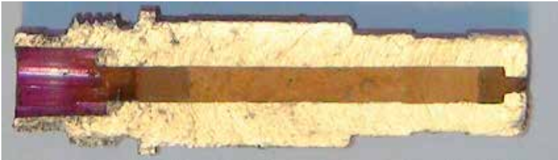
Figure 2. Longitudinal, half cross section of tested multi-segment delay element before its firing.
