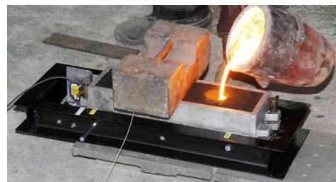
Fig. 4. Pouring of the mould for study of linear shrinkage using laser technology
