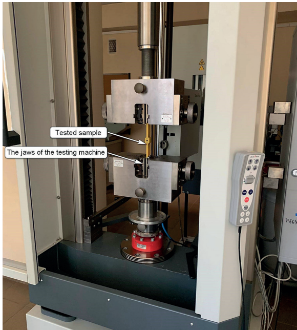
Fig. 4. Testing machine ZWICK/ROELL Z150 with investigated sample mounted in the jaws
