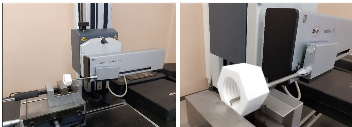
Fig. 4. Measure the nut profile using the MarSurf XC 20
