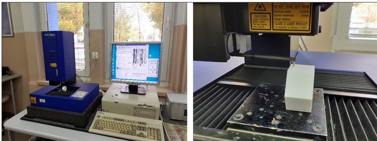
Fig. 5. Surface topography assessment using the TalyScan 150
