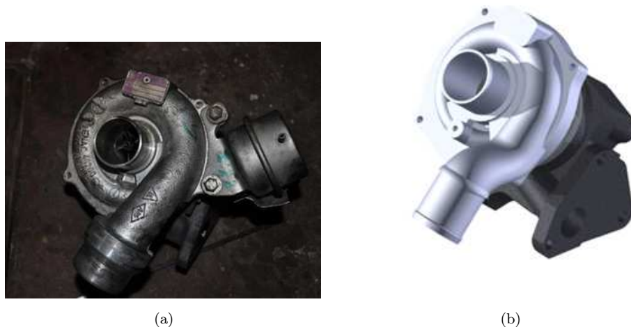
Figure 2: Turbocharger used in the studies: (a) – photograph , (b) – 3D model.
