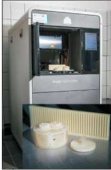
Figure 1: The printer that uses MJP technology, which is situated in a laboratory at the Szewalski Institute of Fluid-Flow Machinery PAS [8].
