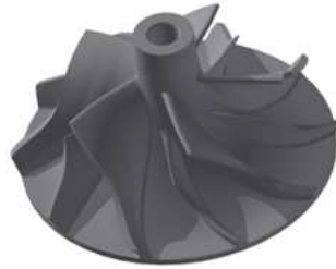
Figure 3: Turbine wheel which is a component of the tested turbocharger.
