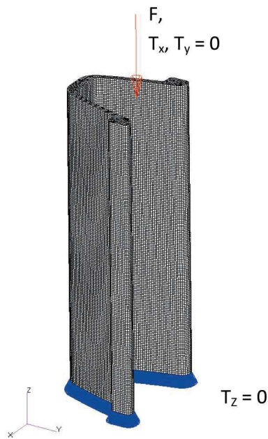
Fig. 16. Boundary conditions in computational model
