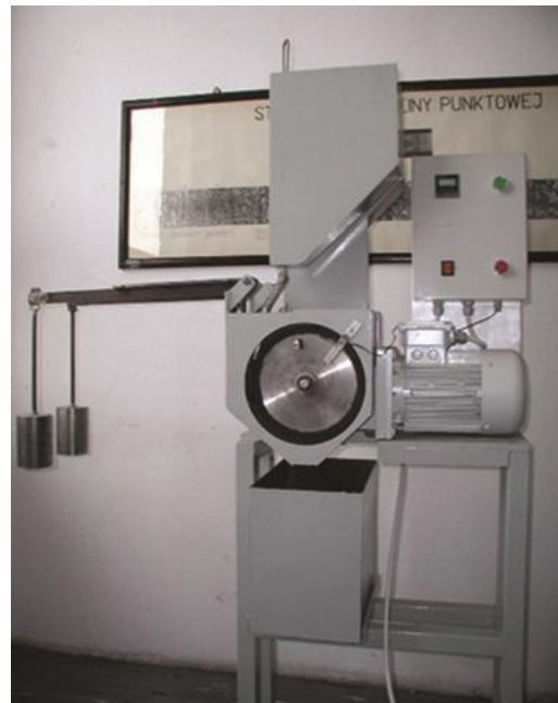
Fig. 4. Abrasive wear test stand according to ASTM G65-00, Procedure A: 1 – abrasive container, 2 – sample holders, 3 – weights, 4 – rubber wheel, 5 – abrasive
