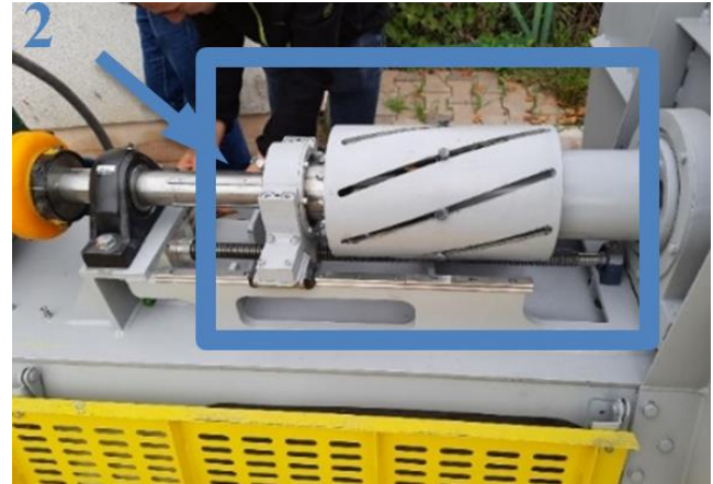
Fig. 31. Steering mechanism forcing a change in rotor geometry on the prototype impeller
