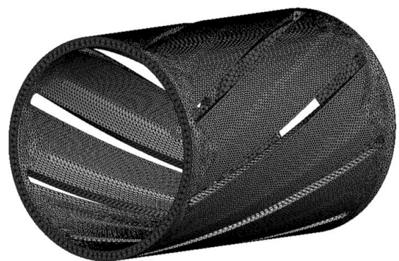
Fig. 10. Mesh generated on the geometrical model of the adjusting drum
