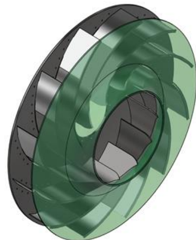
Fig. 4. Geometrical model of the centrifugal fan impeller with the movable blade in maximal position
