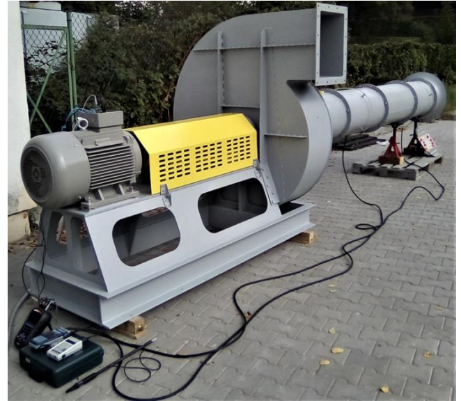
Fig. 33. Standardised airway system during measurements of the prototype fan
