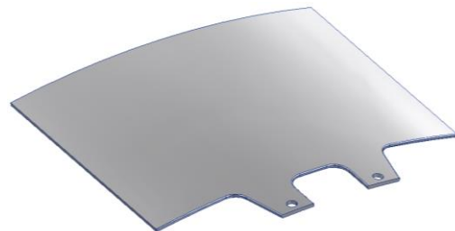
Fig. 8. Final form of the geometrical shape of the movable blade
