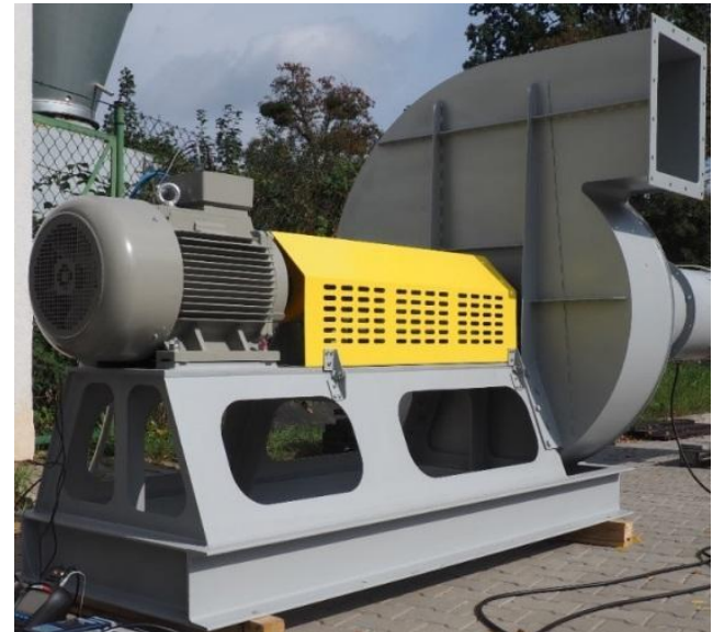
Fig. 32. Prototype of the centrifugal fan with variable impeller geometry
