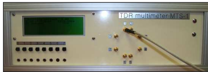
Fig. 2. The measuring device, MTS-1 multimeter
