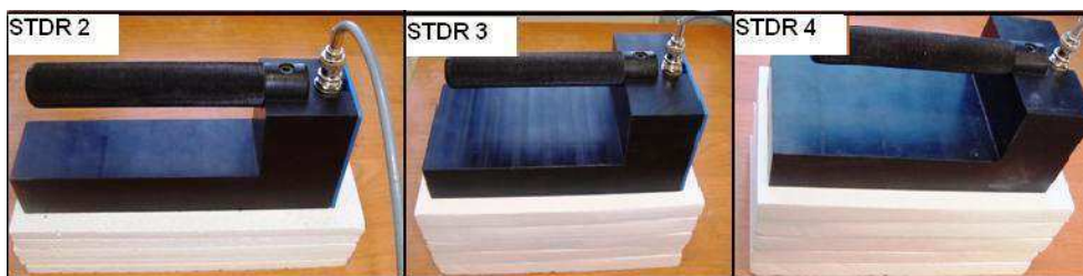
Fig. 1. The surface probes applied to the measurement of the aerated autoclaved concrete (left side) and insulated silicate (middle and right side) moisture
