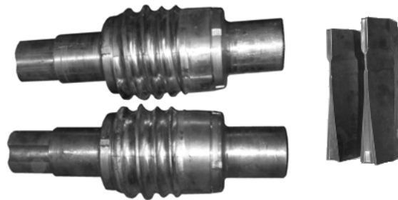
Fig. 7. Rolls with helical wedges (left) and guiding blades (right) used in experimental tests of HWR of balls with diameter of 33mm
