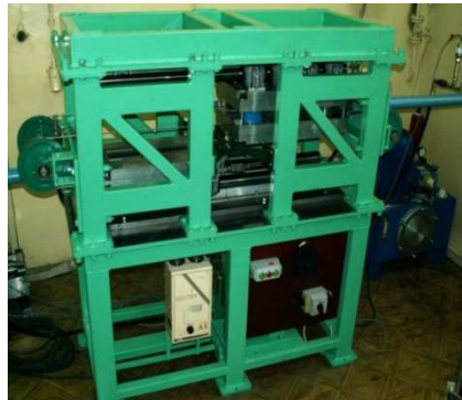
Fig. 3. Flat wedge rolling mill LUW-2 used at Lublin University of Technology
