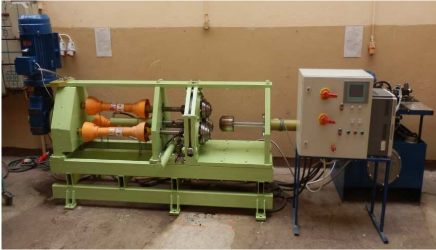
Fig. 10. Rolling extrusion aggregate PO-2 used at Lublin University of Technology
