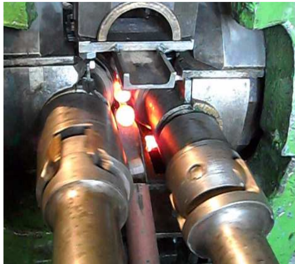
Fig. 8. Way of placing tools in HWR of balls formed at AGH UST in Cracow
