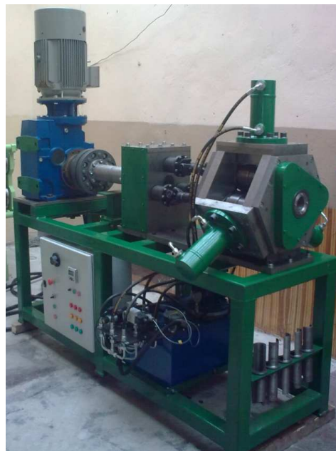
Fig. 13. Prototype aggregate for rotary compression process
