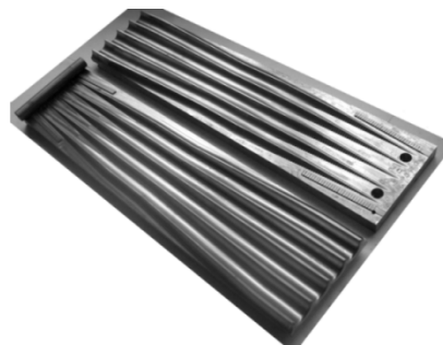
Fig. 4. Billet and the wedge tools used in the tests of multi-wedge rolling of the balls with a diameter of 22mm
